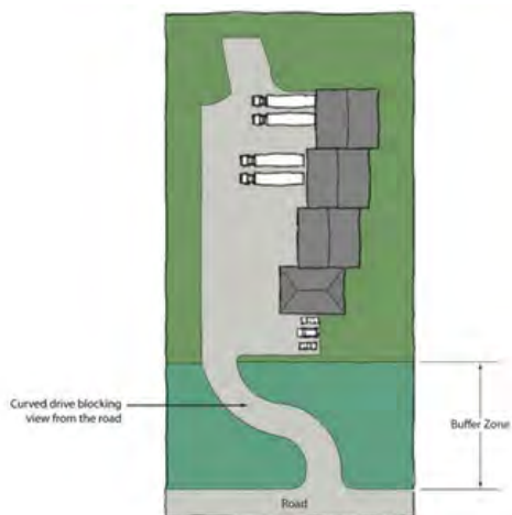
Orienting the narrow façade toward the street, offsetting modular buildings, and maintaining a deep buffer with a meandering driveway can reduce the visual impact of industrial buildings. Source: Cape Cod Commission
