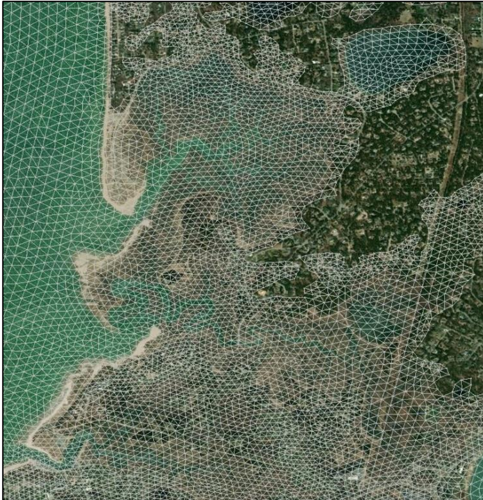
Figure 14. Sample MC-FRM model grid in the Town of Eastham, MA.
